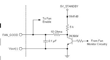
Figure A: Fan status output / Fan enable input interface circuitry.
