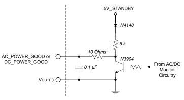
Figure B: Power good interface circuitry.
