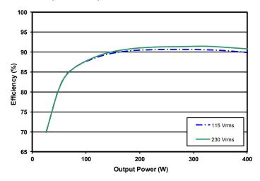
Figure 7: 48  $V_{OUT}$  efficiency curves.
