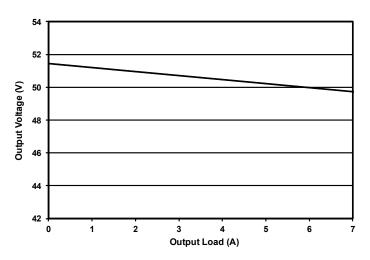
Figure 8: 48  $V_{\rm OUT}$  droop characteristic.
