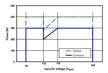
Figure 10: Rated output power vs Input AC Voltage
