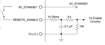
Figure C: Remote enable interface circuitry.
