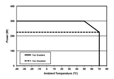
Figure 9: Continuous power derating curve in natural convection.
